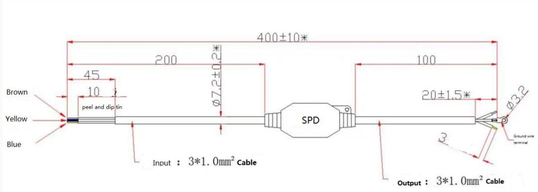
AC input cable length 200mm, three-core 3\*1.0<sup>2</sup>, stripping length 45mm± 5mm, tinning length 10mm;
